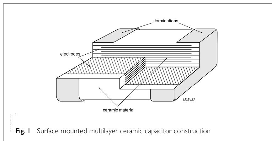
Fig. I Surface mounted multilayer ceramic capacitor construction
