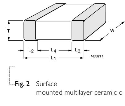
Fig. 2 Surface mounted multilayer ceramic c
