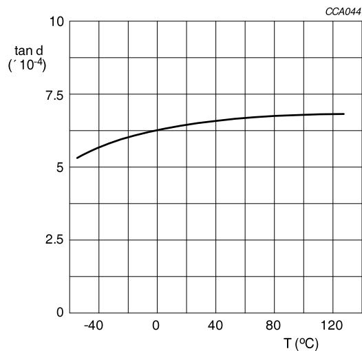
Fig. 5 Typical  $\tan \delta$  as a function of temperatureSOLDERING RECOMMENDATION
